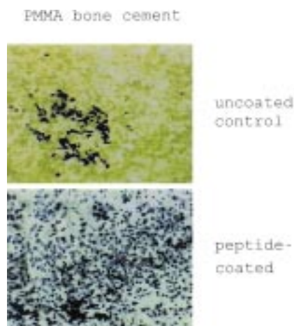
Figure 9. Optical microscopy image of MC3T3-H1 mouse osteoblasts (dark) attached on uncoated PMMA surfaces (top) and on PMMA bone cement treated with acrylamide peptide P6 (bottom). The peptide concentration in the coating solution was 100 \mu\text{M} . While the lower image is representative for the coated surface, the upper image shows the only area of the untreated surface where cell adhesion was observed at all.
