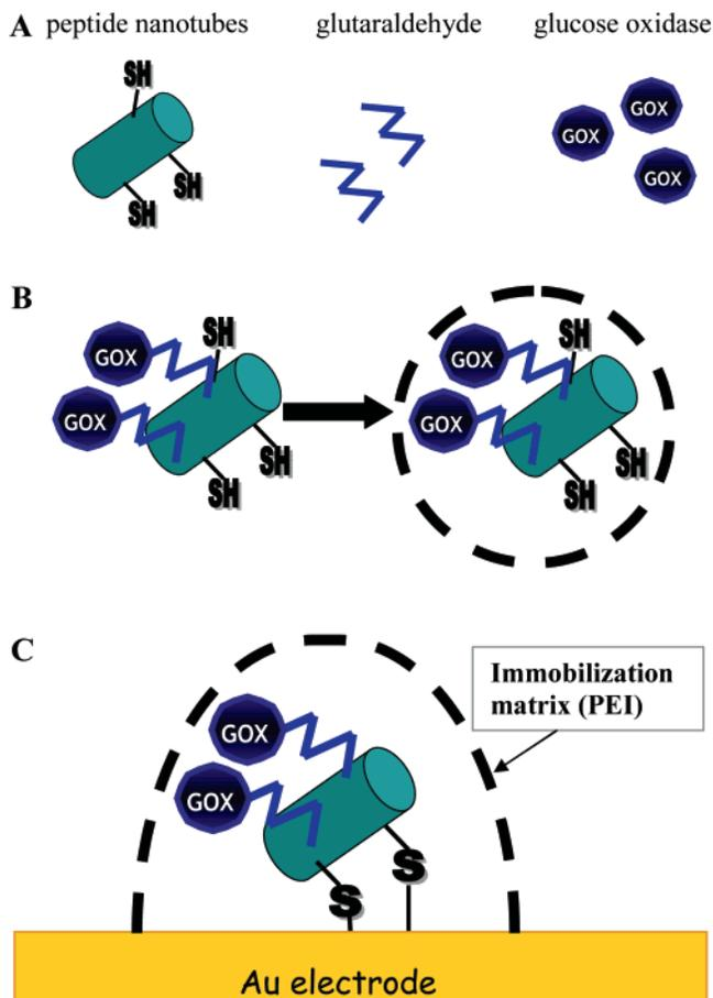
**Figure 4.** Schematic illustration of the procedure used for fabricating the peptide nanotube-based enzymatic electrodes. (A) Thiol-modified peptide nanotubes were mixed with 1  $\mu\text{M}$  GOx in the presence of 0.25% GA. (B) 0.05% PEI was added to the solution. (C) The resulting enzyme-coated peptide nanotubes were deposited on the gold electrode surface and dried at room temperature. (Drawings are not to scale.)
