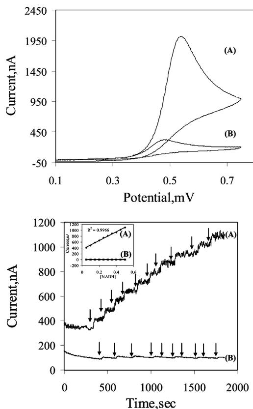
**Figure 2.** Direct measurement of NADH on the peptide nanotube-based electrode. (Top) Cyclic voltammetry of (A) peptide nanotube-based electrode; (B) unmodified electrode measured in a solution containing 50 mM NADH. Scan rate, 50 mV/s. (Bottom) Amperometric response to successive additions of 50  $\mu\text{M}$  NADH. at 0.4 V vs SCE. (A) Peptide nanotube-based electrode; (B) bare electrode. Arrows indicate the addition of increasing concentrations of NADH.
