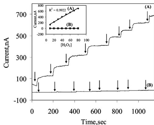
**Figure 1.** Amperometric response to successive additions of 10 mM  $\text{H}_2\text{O}_2$  at +0.4 V vs SCE: (A) peptide nanotube-based electrode; (B) bare electrode. Arrows indicate additions of increasing concentrations of hydrogen peroxide. Inset: a calibration plot illustrating the linear electrode response to hydrogen peroxide addition.
