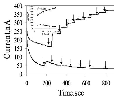
**Figure 6.** Amperometric response to successive additions of 20  $\mu\text{M}$  ethanol to a solution containing 2 mM  $\text{NAD}^+$  and 30 units of ADH (One unit will convert 1.0  $\mu\text{mol}$  of ethanol to acetaldehyde per min at 25  $^\circ\text{C}$  (pH 8.8)). (A) Peptide nanotube-modified electrode; (B) unmodified electrode, 0.1 M phosphate buffer, 0.1 M KCl (pH 8), electrode potential +0.6 V vs SCE. Arrows indicate additions of increasing concentrations of ethanol.
