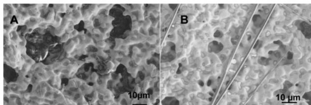
**Figure 3.** SEM images of (A) control gold electrode and (B) peptide nanotube-modified gold electrode.
