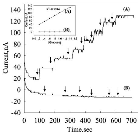
**Figure 5.** Amperometric response to successive additions of 0.2 mM  $\beta$ -D-glucose, measured at 0.6 V vs SCE. (A) Glucose oxidase and peptide nanotube-coated electrode. (B) Glucose oxidase, no nanotube electrode, 0.1 M phosphate buffer solution, 0.1 M KCl (pH 7.5). Arrows indicate the addition of increasing concentrations of glucose.
