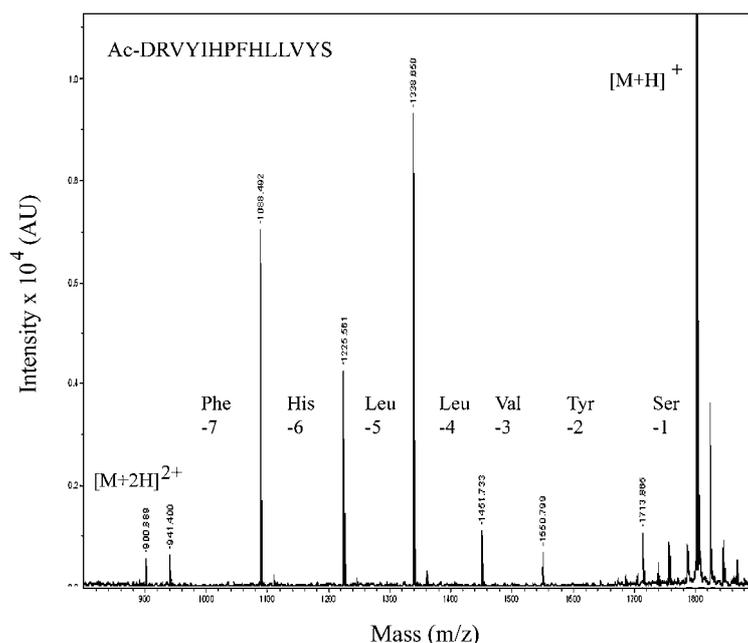
**Fig. 6.** MALDI-TOF Spectrum of C-Terminal Ladder Sequencing of *N*-Acetyl-renin Substrate by TNA1\_CP.
