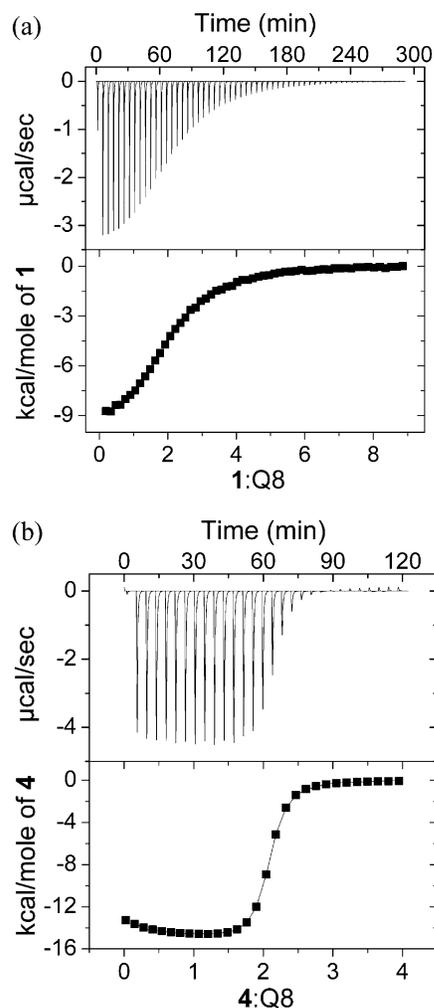
**Figure 3.** ITC data for (a) peptide **1** and (b) peptide **4** at 27 °C in 10 mM sodium phosphate (pH 7.0). Peptide **1** was titrated at 1 mM into a 0.05 mM solution of Q8. Peptide **4** was titrated at 2 mM into a 0.1 mM solution of Q8. At top is the raw data for power versus time. At bottom are integrated enthalpy values versus the molar ratio of peptide:Q8. These data were fit to the “sequential binding model” using Origin 7.0 software.
