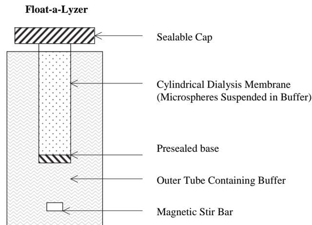
**Figure 1.** Illustration of set-up for in vitro release from microspheres using the Float-a-Lyzer.
