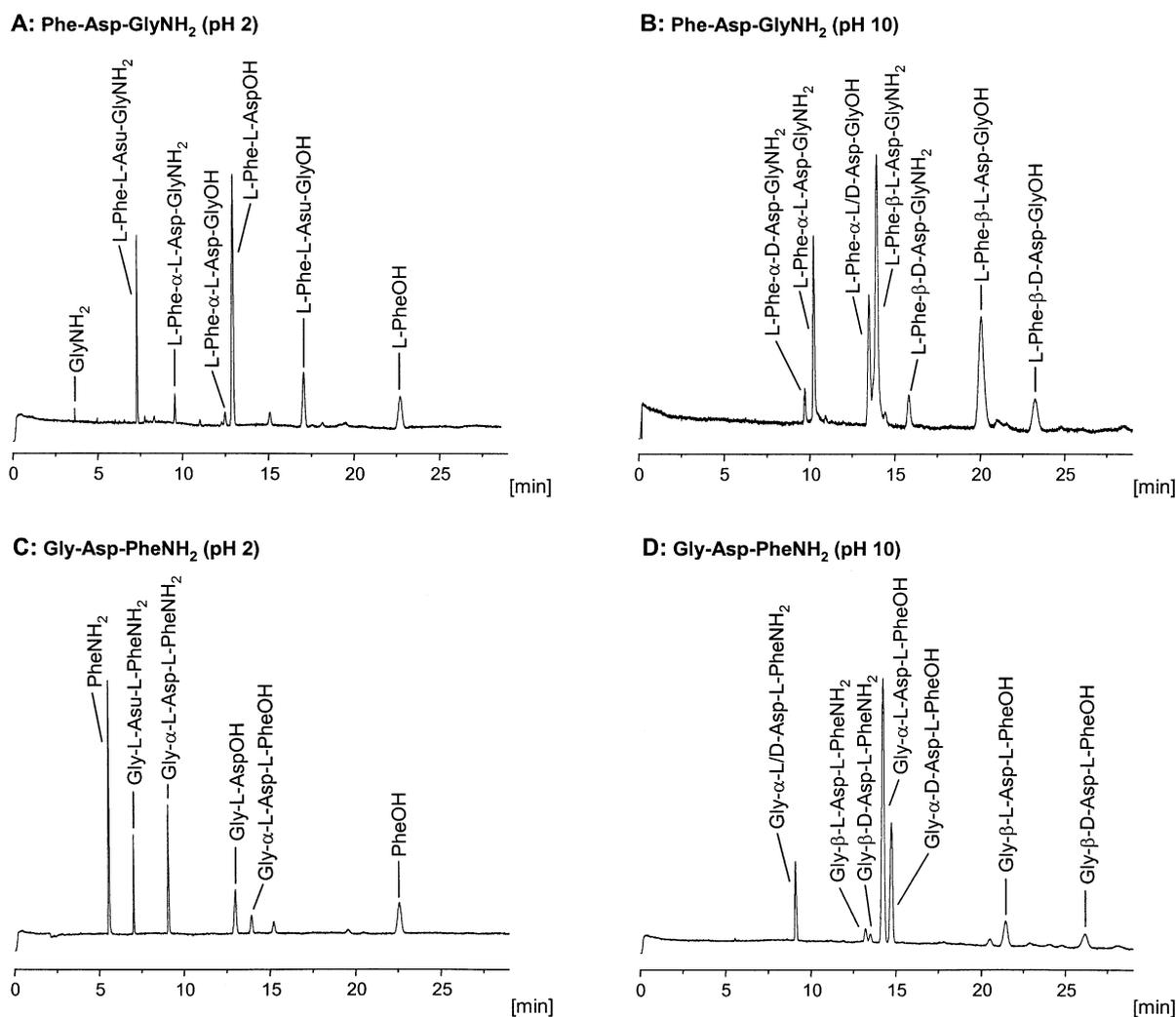
Fig. 5. Electropherograms of Phe-Asp-GlyNH<sub>2</sub> incubated at pH 2 for 31 h (A) and at pH 10 for 24 h (B) and of Gly-Asp-PheNH<sub>2</sub> incubated at pH 2 for 48 h (C) and at pH 10 for 72 h (D). Conditions: 50 mM phosphate buffer, pH 3.0, 47/40 cm capillary, 50 mM i.d., UV detection at 215 nm, 23 kV.
