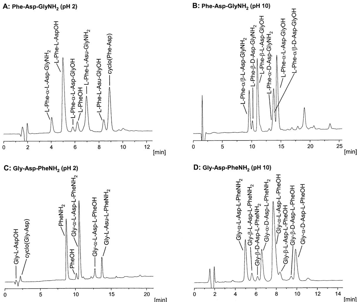
Fig. 2. Chromatograms of Phe-Asp-GlyNH<sub>2</sub> incubated at pH 2 for 24 h (A) and at pH 10 for 48 h (B) and of Gly-Asp-PheNH<sub>2</sub> incubated at pH 2 for 24 h (C) and at pH 10 for 48 h (D). Conditions: mobile phase gradient 7–20% B within 15 min (A), 2–13% B within 30 min (B), 1–20% B within 10 min (C) and 10–20% B within 15 min (D). Eluent A was 0.1% TFA in water and eluent B was 0.1% TFA in water–acetonitrile (5:95, v/v). Flow 0.2 ml/min. Detection at 215 nm.
