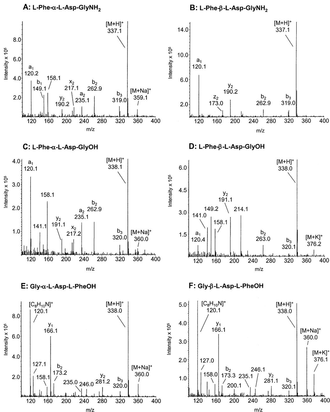
Fig. 4. Mass spectra of L-Phe- $\alpha$ -L-Asp-GlyNH<sub>2</sub> (A), L-Phe- $\beta$ -L-Asp-GlyNH<sub>2</sub> (B), L-Phe- $\alpha$ -L-Asp-GlyOH (C), L-Phe- $\beta$ -L-Asp-GlyOH (D), Gly- $\alpha$ -L-Asp-L-PheOH (E) and Gly- $\beta$ -L-Asp-L-PheOH (F). (A) and (B) were analyzed by injection of reference substances, (C)–(F) were recorded from samples of Phe-Asp-GlyNH<sub>2</sub> and Gly-Asp-PheNH<sub>2</sub> after incubation at pH 10.
