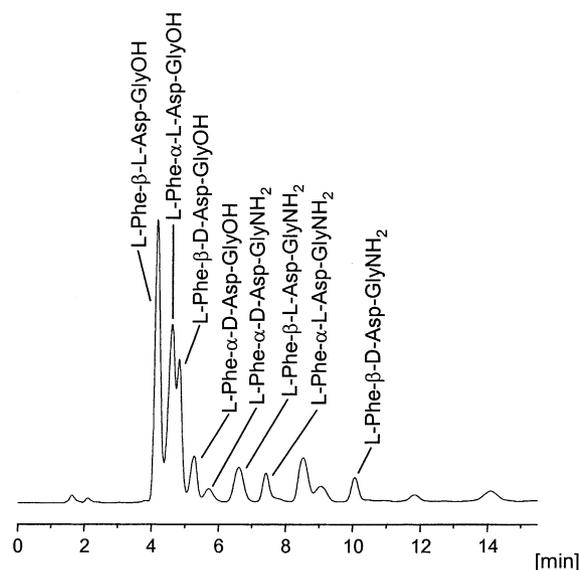
Fig. 3. Chromatogram of Phe-Asp-GlyNH<sub>2</sub> incubated at pH 10 for 48 h analyzed in phosphate buffer with a gradient of 2–13% of eluent B in 30 min. Eluent A was 15 mM aqueous phosphate, pH 5.0, and eluent B was water–acetonitrile (5:95, v/v). Flow 0.2 ml/min. Detection at 215 nm.
