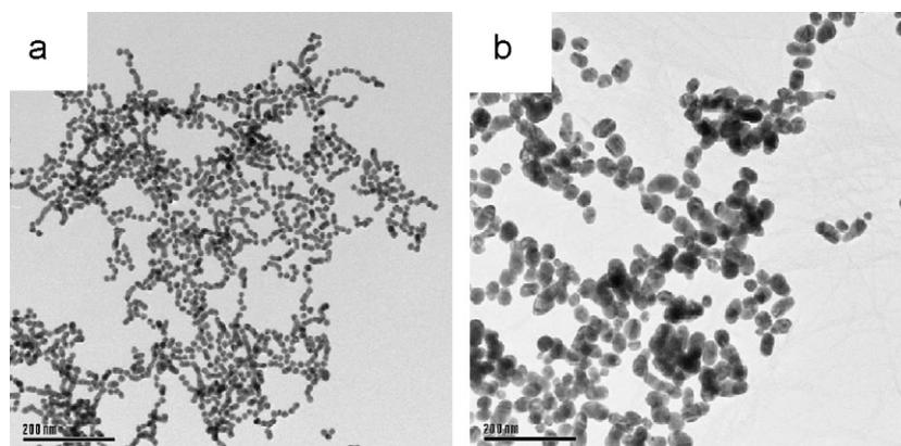
**Fig. 4.** TEM micrograph of the flocculated Au nanoparticles resulted from modification with amino acids: (a) 13 nm Au nanoparticles modified with  $1.0 \times 10^{-2}$  M Arg and (b) 35 nm Au nanoparticles conjugated with  $1.0 \times 10^{-3}$  M Cys.
