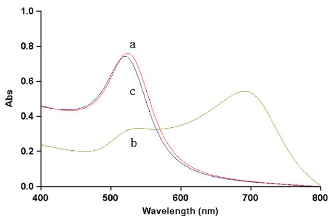
**Fig. 5.** UV-vis spectra of 13 nm Au nanoparticles capped with BSA: (a) unmodified Au nanoparticles, (b) unmodified Au nanoparticles after 10% NaCl addition and (c) BSA-capped Au nanoparticles after 10% NaCl addition.
