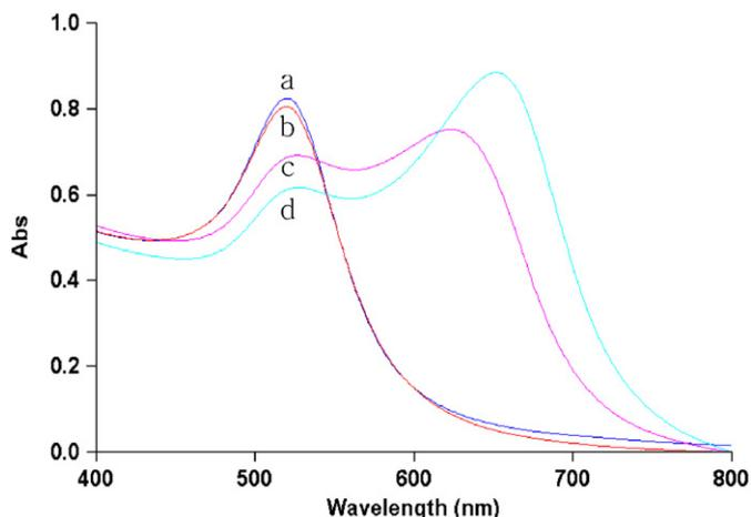
**Fig. 2.** UV-vis spectra of 13 nm Au nanoparticles conjugated with different concentrations of Arg: (a) unmodified Au nanoparticles, (b) Au nanoparticles conjugated with  $1.0 \times 10^{-3}$  M Arg, (c) Au nanoparticles conjugated with  $5.0 \times 10^{-3}$  M Arg and (d) Au nanoparticles conjugated with  $1.0 \times 10^{-2}$  M Arg.
