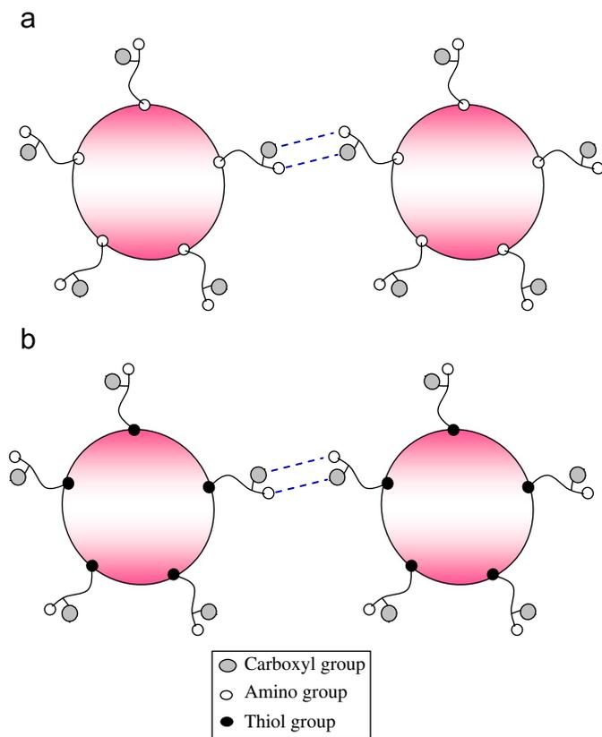
**Fig. 3.** Illustration of the assembly of Arg-modified Au nanoparticles (a) and Cys-modified Au nanoparticles (b) induced by hydrogen bonding between amino acid molecules in adjacent Au nanoparticles.
