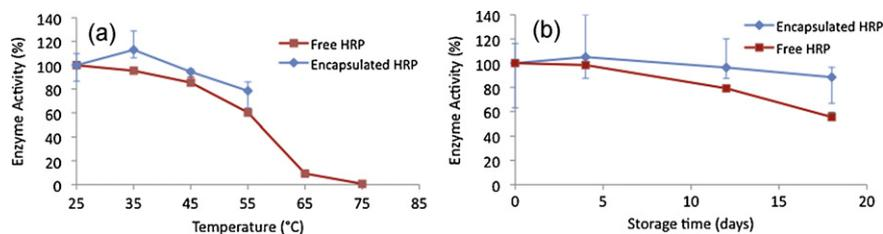
Fig. 4. (a) Thermal stability of the encapsulated HRP. (b) Storage stability of the encapsulated HRP.
