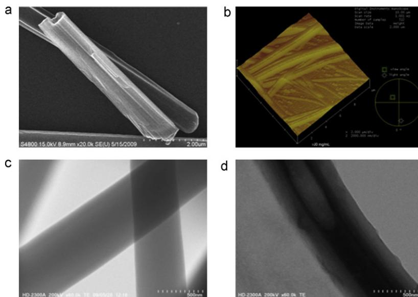
**Fig. 1.** (a) SEM image of the PNT, (b) AFM image of the PNT, (c) STEM image before the encapsulation of the HRP inside the PNT, and (d) after the encapsulation.
