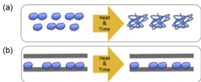
**Fig. 5.** Schematics of possible explanation how the enzyme can be protected by the PNT encapsulation at high temperature and for an extended storage time. (a) Free HRP. (b) Encapsulated HRP.
