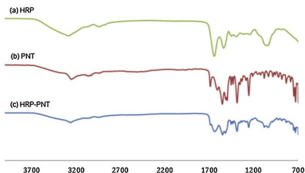
Fig. 3. ATR-FTIR spectra of (a) free HRP, (b) PNT and (c) the encapsulated HRP into the PNT.
