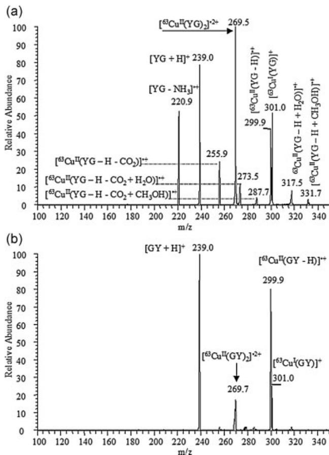
**Figure 5.** CID spectra of  $[\text{Cu}^{\text{II}}(\text{M}_a)(\text{M}_b)]^{*2+}$ : (a)  $\text{M}_a = \text{M}_b = \text{YG}$  and (b)  $\text{M}_a = \text{M}_b = \text{GY}$  at relative collision energy of 7%. The bold arrow indicates the precursor ion.
