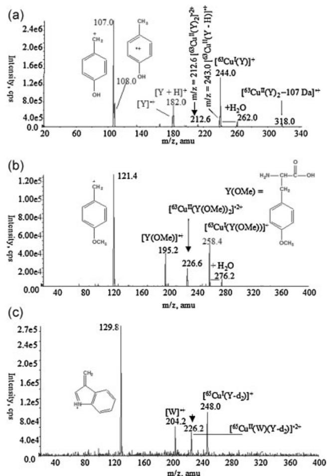
**Figure 1.** CID spectra of (a)  $[\text{Cu}^{\text{II}}(\text{Y})_2]^{\bullet 2+}$ , (b)  $[\text{Cu}^{\text{II}}(\text{Y}(\text{OMe}))_2]^{\bullet 2+}$ , and (c)  $[\text{Cu}^{\text{II}}(\text{W})(\text{Y-d}_2)]^{\bullet 2+}$  all at  $E_{\text{lab}} = 7$  eV. The use of the  $^{65}\text{Cu}$ -containing complex and the  $\text{d}_2$  amino acid of  $\text{Y}$  in (c) was necessitated by isobaric interferences. The bold arrow indicates the precursor ion.
