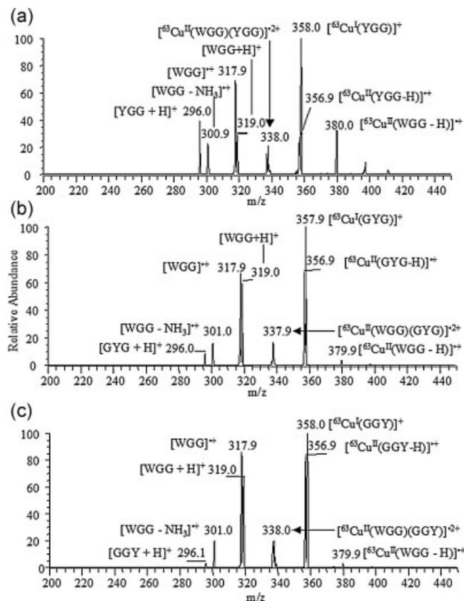
**Figure 7.** CID spectra of complexes of  $[\text{Cu}^{\text{II}}(\text{M}_a)(\text{M}_b)]^{2+}$  where (a)  $\text{M}_a = \text{WGG}$  and  $\text{M}_b = \text{YGG}$ ; (b)  $\text{M}_a = \text{WGG}$  and  $\text{M}_b = \text{GYG}$ ; and (c)  $\text{M}_a = \text{WGG}$  and  $\text{M}_b = \text{GGY}$  at relative collision energy 7%. The bold arrow indicates the precursor ion.
