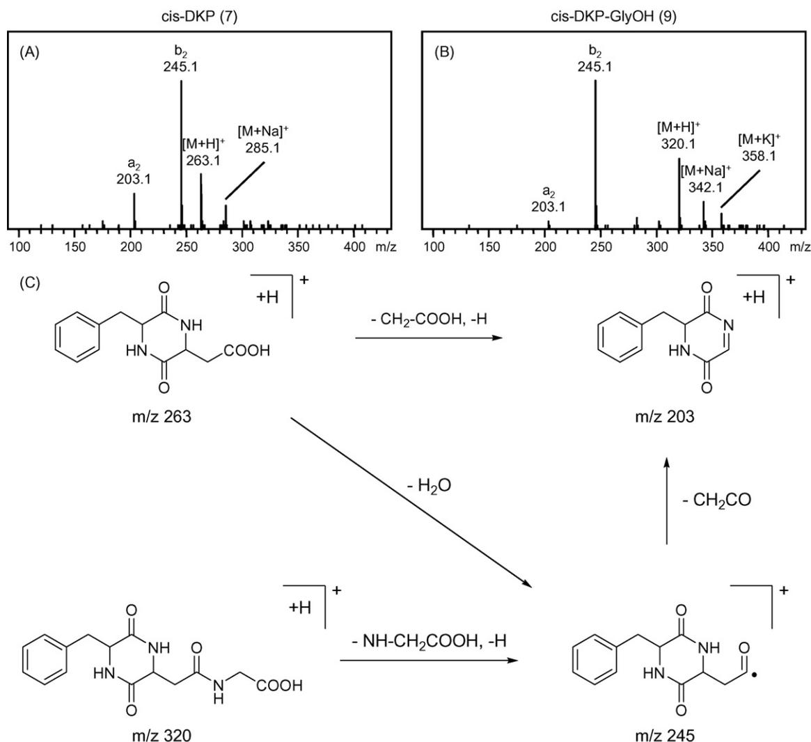
**Fig. 3.** Mass spectra of diketopiperazine derivatives (A and B) and proposed fragmentation pattern (C).
