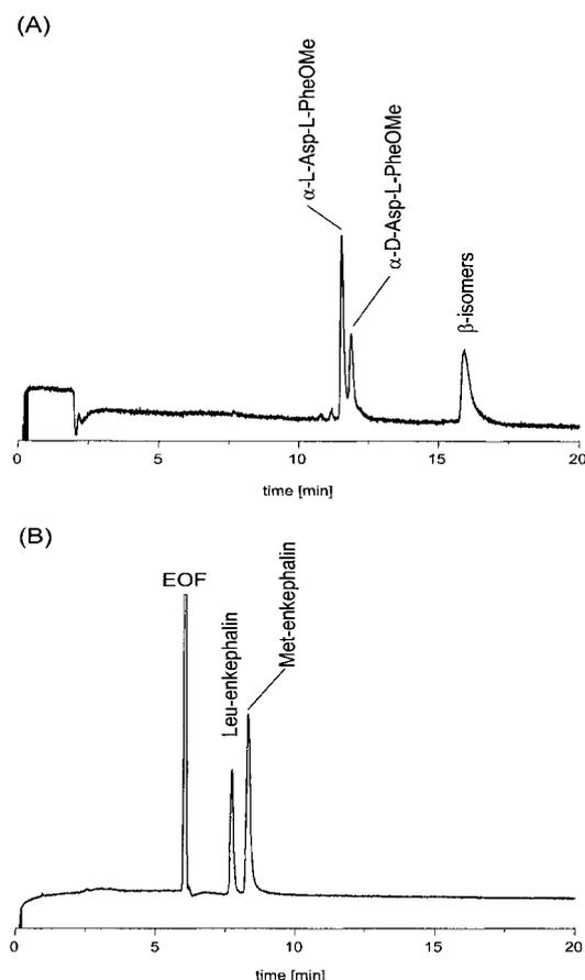
**Figure 5.** Electropherograms of  $\alpha/\beta$ -DL-Asp-L-PheOMe and of the enkephalins obtained in methanol. (A)  $\alpha/\beta$ -DL-Asp-L-PheOMe in 28 mM borate buffer  $\text{pH}_{\text{app}}$  10.3; applied voltage, –25 kV; (B) Met- and Leu-enkephalin in 25 mM acetate buffer  $\text{pH}_{\text{app}}$  7.0; applied voltage, +25 kV.
