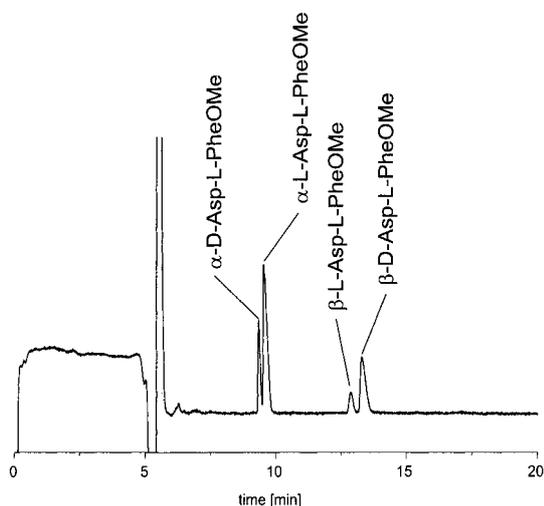
**Figure 4.** Separation of the  $\alpha/\beta$ -DL-Asp-L-PheOMe diastereomers in methanolic dichloroacetate buffer. 25 mM dichloroacetate buffer  $\text{pH}_{\text{app}}$  3.8; applied voltage, +25 kV.
