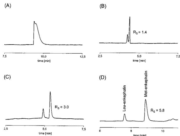
**Figure 6.** Effect of pH on the resolution of Met- and Leu-enkephalin in methanol. (A) 25 mM trichloroacetate buffer  $\text{pH}_{\text{app}}$  2.2, (B) 25 mM chloroacetate buffer  $\text{pH}_{\text{app}}$  4.4, (C) 25 mM chloroacetate buffer  $\text{pH}_{\text{app}}$  5.1, (D) 25 mM acetate buffer  $\text{pH}_{\text{app}}$  5.7. Applied voltage, +25 kV.
