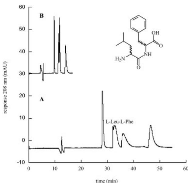
**Figure 5.** Chiral separation of Leu-Phe on TAG by CEC using different mobile phases,  $U = 15$  kV; (A) TEAA, pH 4.1/ACN (80:20),  $U = 15$  kV; (B) TEAA, pH 4.1/ACN (70:30),  $U = 28$  kV.
