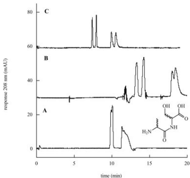
**Figure 4.** Chiral separation of Ala-Ser on TAG by CEC using different mobile phases,  $U = 15$  kV. (A) TEAA, pH 4.1/ACN (90:10); (B) TEAA, pH 4.1/ACM/MeOH (50:30:20); (C) TEAA, pH 4.1/ACN/EtOH (50:30:20).
