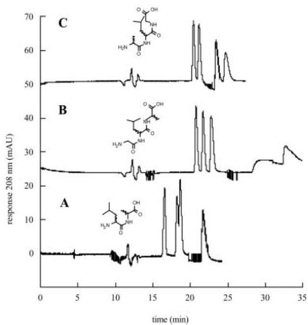
**Figure 6.** Chiral separation of (A) Leu-Ala, (B) Gly-Leu-Ala and (C) Ala-Leu-Gly on TAG by CEC. Mobile phase: TEAA, pH 4.1/ACN/MeOH (50:30:20),  $U=15$  kV.
