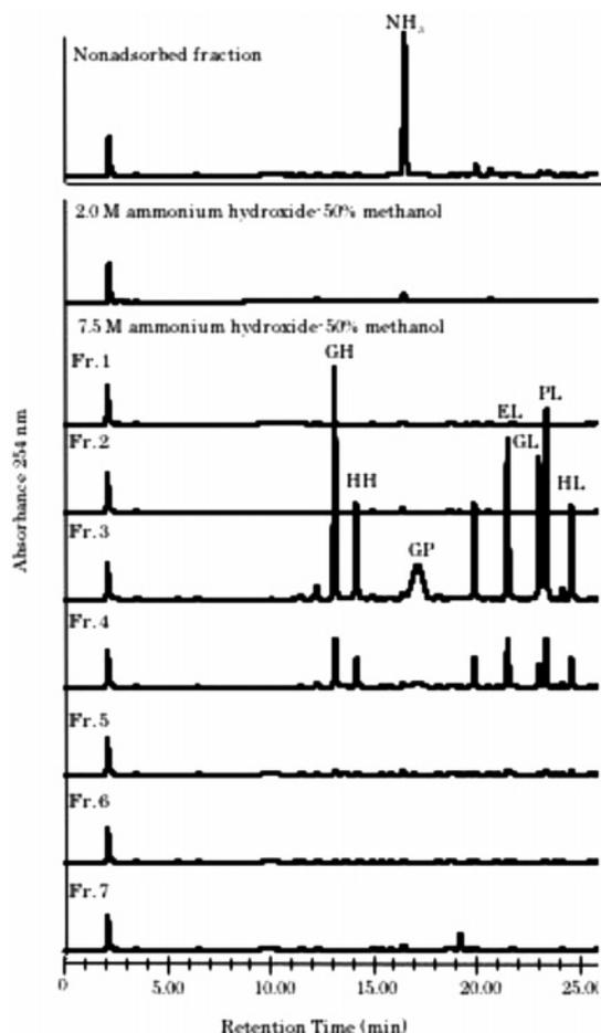
**Figure 3.** Elution of dipeptides from a mini spin column packed with a strong cation exchanger (AG 50WX-8W). Twenty nanomoles of the authentic peptides was loaded onto a mini spin column and successively eluted with 200  $\mu$ L of 2.0 and 7.5 M ammonium hydroxide containing 50% methanol. Aliquots of fractions were derivatized with PITC and resolved by RP-HPLC by using an ammonium acetate buffer system.
