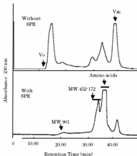
**Figure 4.** Effect of SPE treatment on the chromatogram of the SEC mode. Eight milliliters of the ethanol-soluble fraction with and without SPE pretreatment was loaded onto a Superdex Peptide 10/30 HR column. Key:  $V_o$ , void volume;  $V_m$ , exclusion limit.
