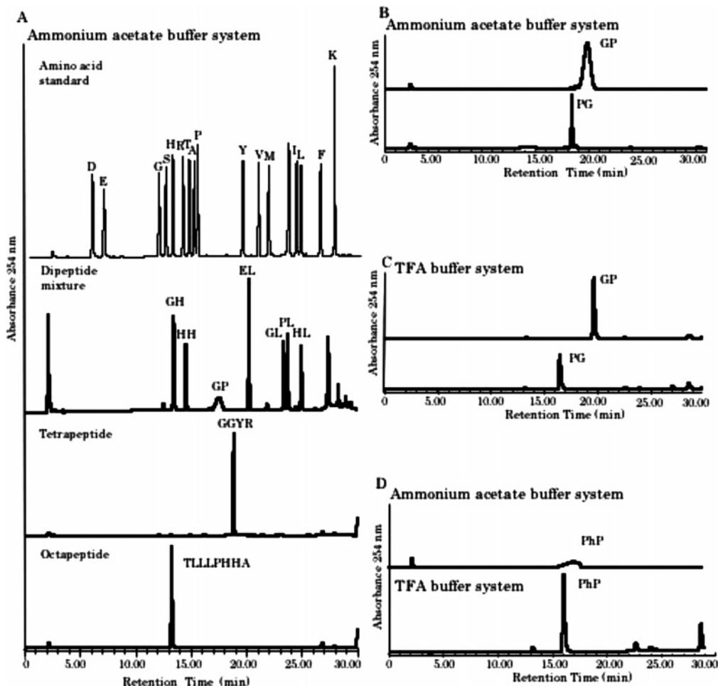
**Figure 2.** Resolution of PTC-peptides and PTC-amino acids. Five hundred picomoles of PTC-amino acids and di-, tetra-, and octapeptides was resolved by RP-HPLC by using an ammonium acetate buffer system, pH 6.0. PTC-Gly-Pro (A), PTC-Pro-Gly (B, C), and PTC-Pro-Hyp (D) were resolved by RP-HPLC by using an ammonium acetate buffer system and a TFA system. PhP means Pro-Hyp. For the TFA system, a 250 mm  $\times$  4.6 mm i.d. column was used.
