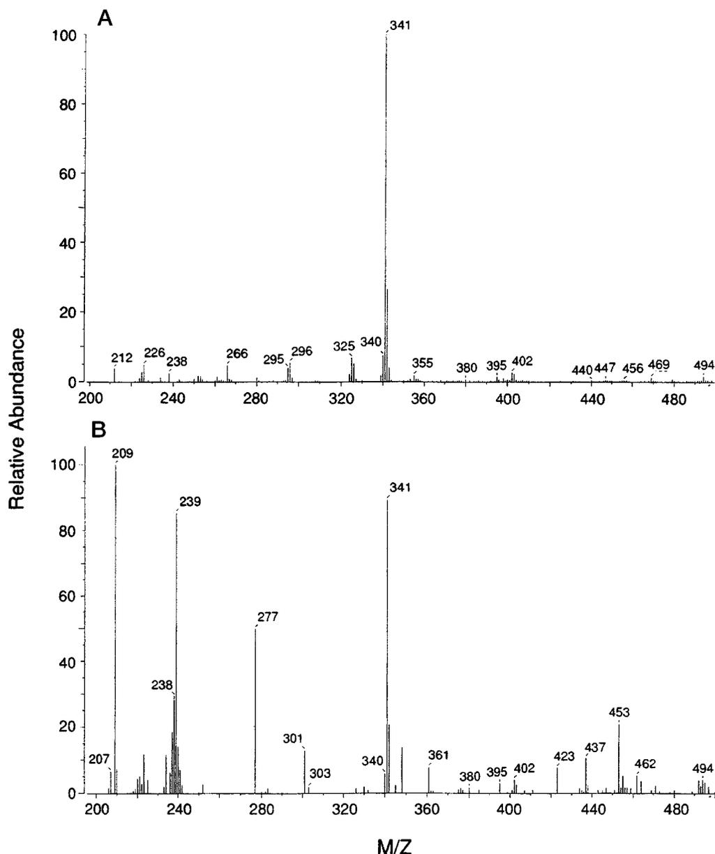
FIG. 6. Liquid chromatography/mass spectrometry analysis of imidazolysine standard (A) and partially purified imidazolysine from human serum proteins (B). The molecular mass for the peak in serum proteins (at the retention time of purified imidazolysine, 15–16 min) was identical to the imidazolysine standard ( $m/z$  341). Background signals were subtracted to remove the mass ions from the matrix and solvent.
