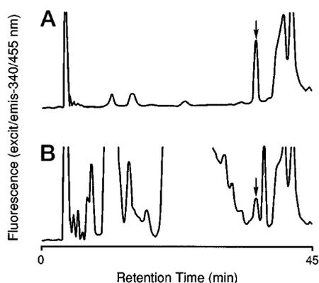
FIG. 5. Representative chromatograms of imidazolysine standard (A) and serum protein hydrolysate (B). Serum proteins were precipitated with 10% trichloroacetic acid and hydrolyzed with 6 N HCl. Serum proteins showed a peak at a retention time identical to that of imidazolysine standard (indicated by arrows). Imidazolysine was quantified in the hydrolysates by two-step HPLC and postcolumn derivatization with OPA. Other details are described under "Experimental Procedures."
