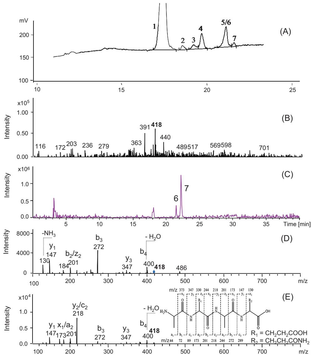
**Fig. 5.** Evaluation of fraction 6 of tandem Gemini C18/Synergi Fusion-RP column: (A) HILIC-CAD chromatogram of fraction 6, (B) scan spectrum of peak 6, (C) extracted ion chromatogram of  $m/z$  418: (6) AlaGlu(AlaGln); (7) AlaGluAlaGln, (D) fragmentation spectrum of AlaGlu(AlaGln), (E) fragmentation spectrum of AlaGluAlaGln peak annotation: 1 Val, 2 unknown, 3 unknown, 4 Pro, 5 AlaGln/6 AlaGlu(AlaGln), 7 AlaGluAlaGln.
