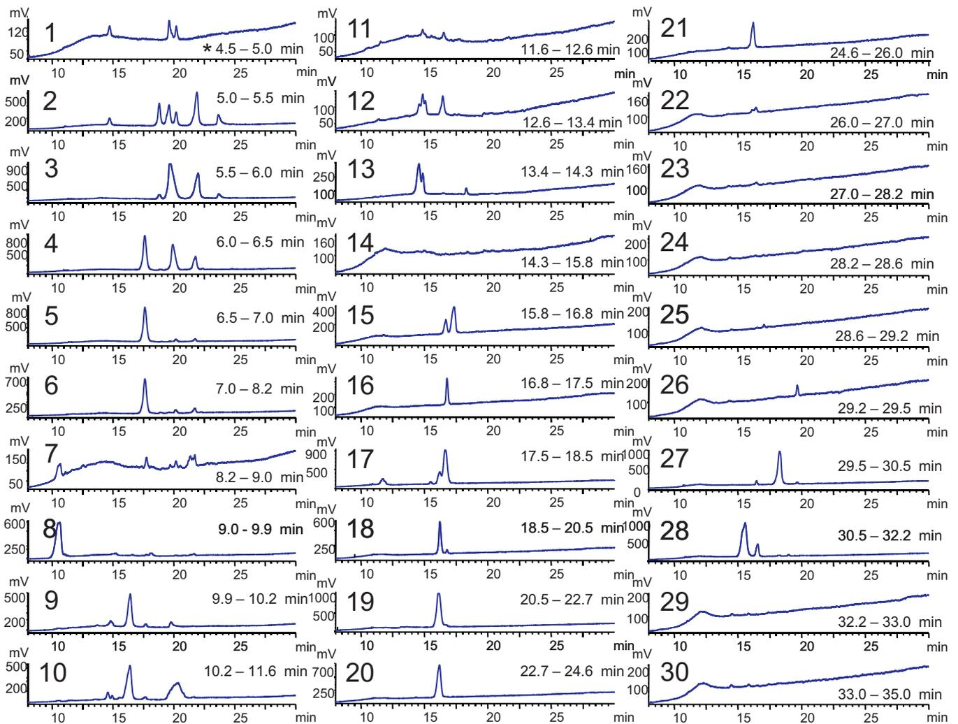
**Fig. 3.** Representative 2nd dimension HILIC chromatograms (step 3) of the 30 collected fractions from the 1st dimension tandem RP column). The chromatograms were recorded with the CAD. The injection volume was 2  $\mu$ l for fractions 1, 2, 16, 18 and 20  $\mu$ l for the remaining fractions. \* Fraction collection time intervals.
