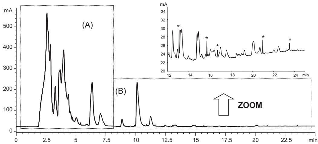
**Fig. 2.** RPLC chromatogram of the stressed formulation recorded with the CAD detector. A Gemini C18 column was employed (step 1). Part (A) contains polar hydrophilic compounds, which were investigated in detail using the multidimensional analysis assay. Part (B) of the chromatogram was directly analyzed using the RPLC method with CAD detection and unified calibration. Peaks denoted with an asterisk are spikes.
