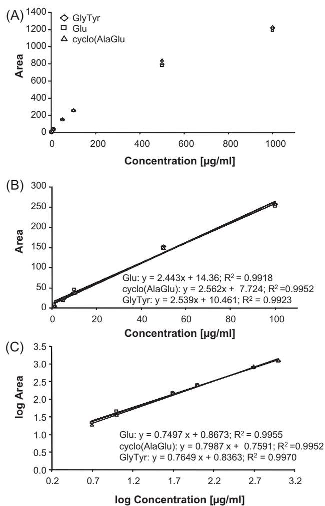
Fig. 4. Calibration curves: entire range (A), linear calibration function (B), double logarithmic over full concentration range (C) of the three compounds Glu, cyclo(AlaGlu) and GlyTyr using the RP method of the first separation step (Gemini C18).
