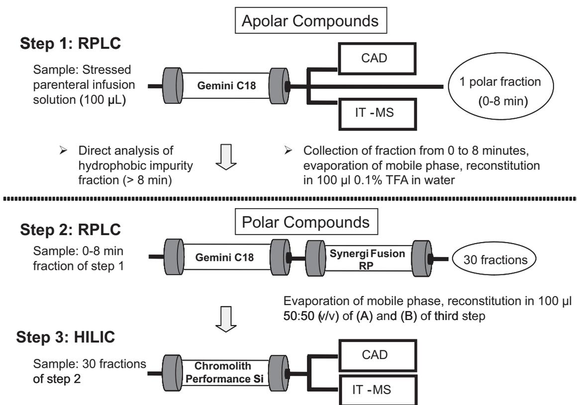
Fig. 1. Scheme of the workflow of the multidimensional analysis assay for establishing the impurity profile of a stressed nutritional infusion solution.
