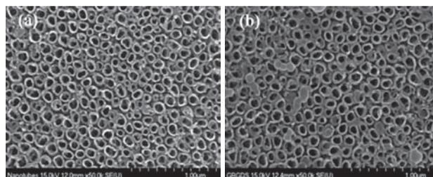
**Figure 1.** FE-SEM images of (×50,000) (a) TiO<sub>2</sub> nanotubes, (b) GRGDS-TiO<sub>2</sub> nanotubes.
