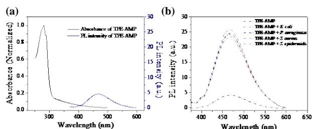
**Fig. 2** (a) UV-visible absorption and PL spectra of TPE-AMP in PBS (pH = 7.4, 0.1 mg/mL) with an excitation wavelength of 350 nm; (b) PL spectra of TPE-AMP in the absence and presence of *E. coli*, *P. aeruginosa*, *S. aureus* and *S. epidermidis* in PBS (pH = 7.4) with an excitation wavelength of 350 nm.
